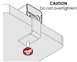
**Screw Down - On surface** (Screw hole is 5mm (0.20"), suitable for < No. 10 screw)
